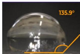
Figure 5: Water contact angle of OP-magnetite
