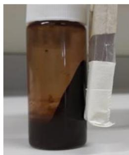
Figure 17: Magnetic property of OP-ferrofluid
