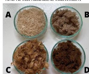
[A] – *in natura* pseudo-stem fiber; [B] – treated pseudo-stem fiber (40% NaOH, 40min autoclaving).
