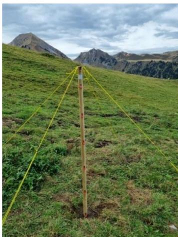
Figure 4: Snow pole (with sensors at heights of 0, 30, 60, 90, 120, 150 and 170 cm)
