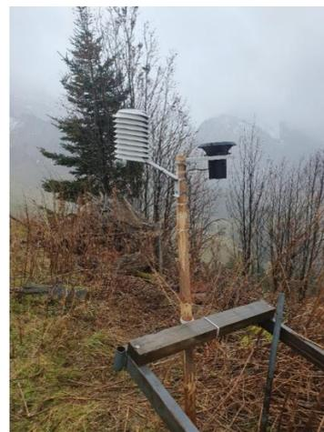
Figure 5: Weather station mounted on a stake
