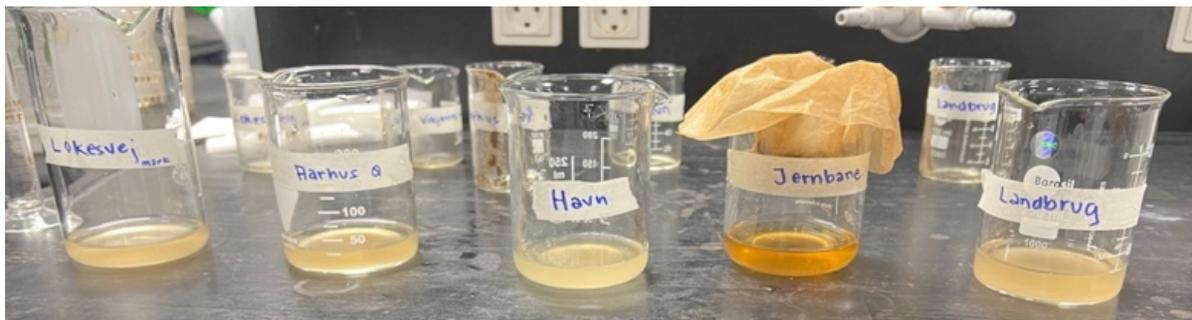
Figure 10: Soil samples after filtration ready for colorimetry analysis, where havn is harbor and jernbane is railway
