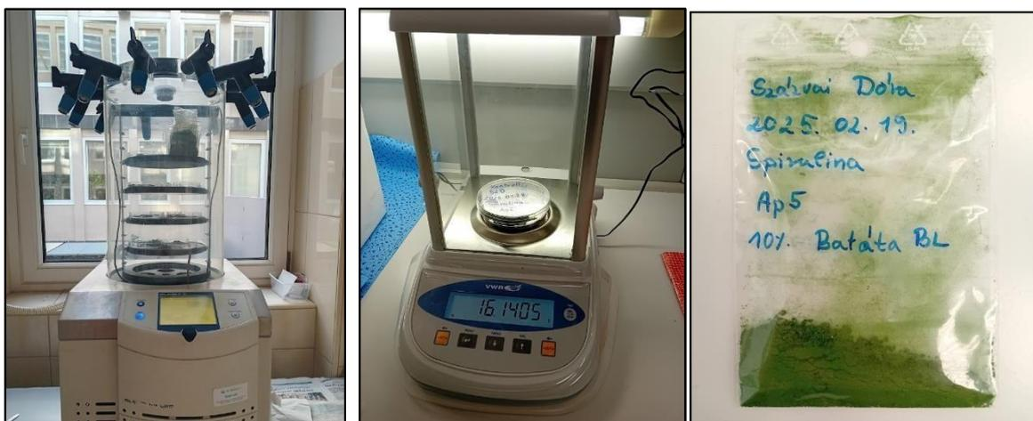
**Figure 12:** Lyophilization, measuring the dry weight of the samples, and dried algae biomass
