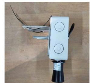
Figure 6: Mounting using brackets and cable ties
