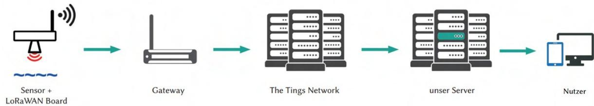
**Figure 8: Schematic and simplified illustration of the individual components and their interconnection within the WarnMe system.**
