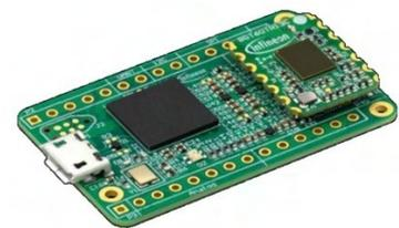
**Figure 7: Development kit for radar based measurement of flow velocity and flow rate.**
