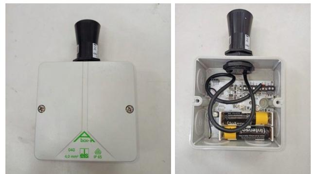
Figure 5: Housing of the ultrasonic sensor, left: closed,
