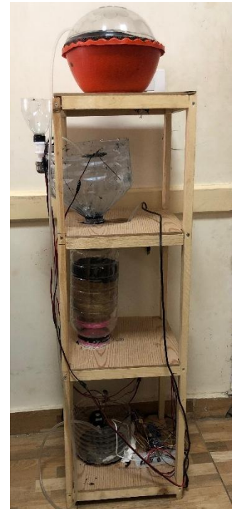
Figure 19. Three stage water treatment system
