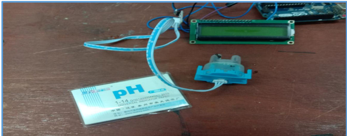
Figure 2.1. Show the Ph Level Tester and Arduino Turbidity Sensor as the tools used to assess the Ph Level and Turbidity of the water.
