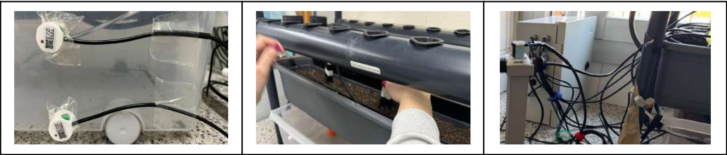
Fig. 28. Water inlet to the leachate tank, regulated by the tank's level sensors (m/m).
