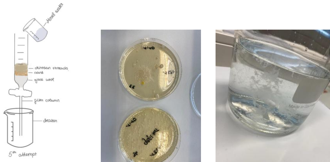
Figure 8: Set-up for Filter Test 5; poor filtration result; filaments in the beaker
